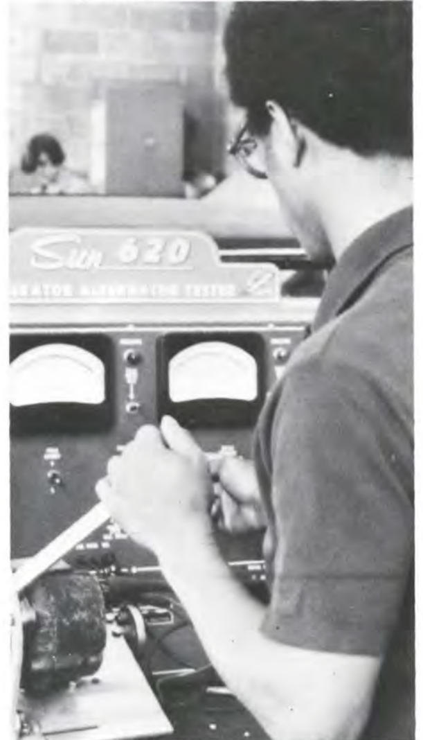
Billy Goodson, President of the Auto Club, tests an electrical flow through the alternator.
