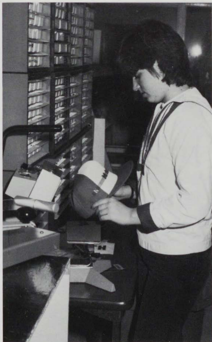
Above: After placing the letters on a tape across the item, Laura places the hat on the heat seal machine. Above Right: Laura then closes the iron and holds the handle down for a few seconds as the heat transfers the letters to the hat.
