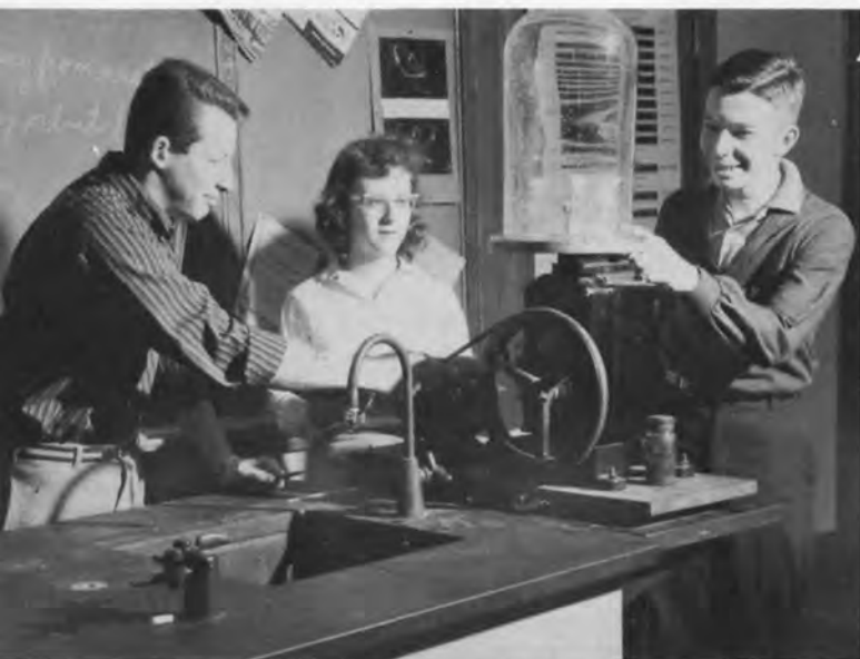
BELOW—Roger Friedlander, Louise Strang, and Edward Ehrenkranz boil water at room temperature with a vacuum pump.
