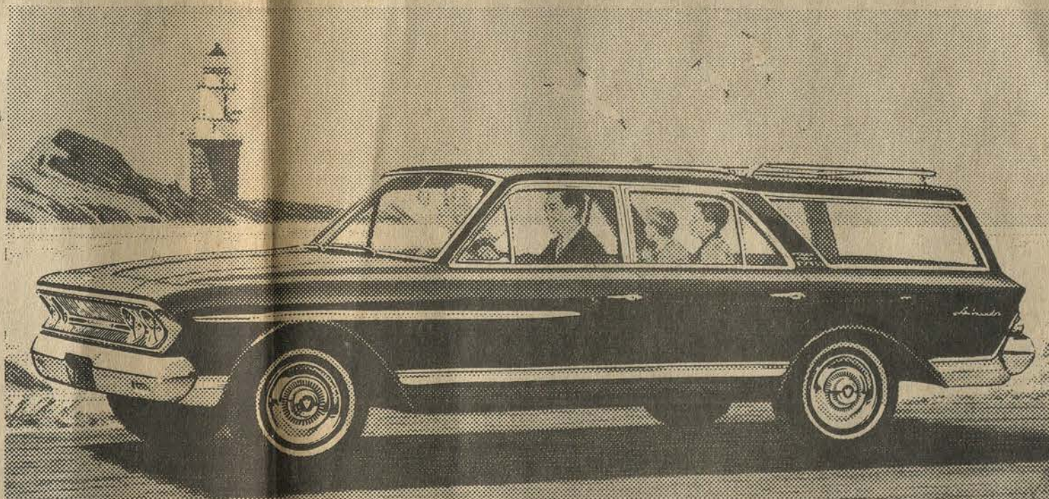
1963 Rambler Ambassador V-8 "990" Wagon. 250 HP standard, 270 HP optional. Lockable hidden compartment in rear.
