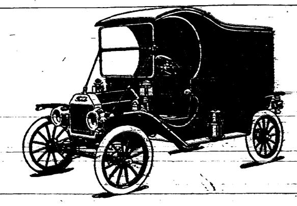
FORE-DOORS DETACHABLE. Pneumatic Cushions, extra roomy tonneau, taper rear axles, enclosed valves, motor 32 x 4, fully equpped with 3 oil lamps; a gas lamps, wind shield, Stewart speedometer, top and curtains, pump, tools, etc. Other Models are
