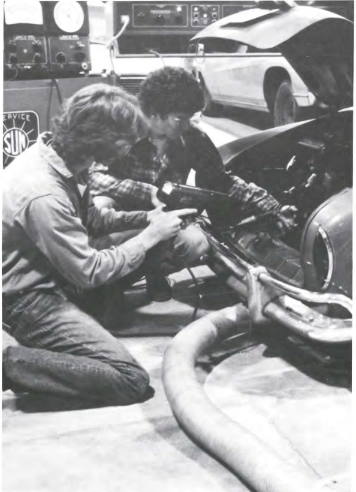
Glen Hendrichs and James Christman tune an engine using a timing light in Mr. Daniel Wainwright's Auto Mechanics class.
