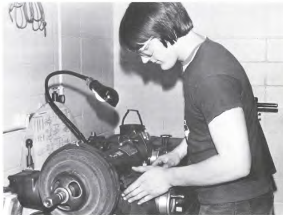
Junior John Ricci grinds a brake drum on a lathe in the Auto Shop.
