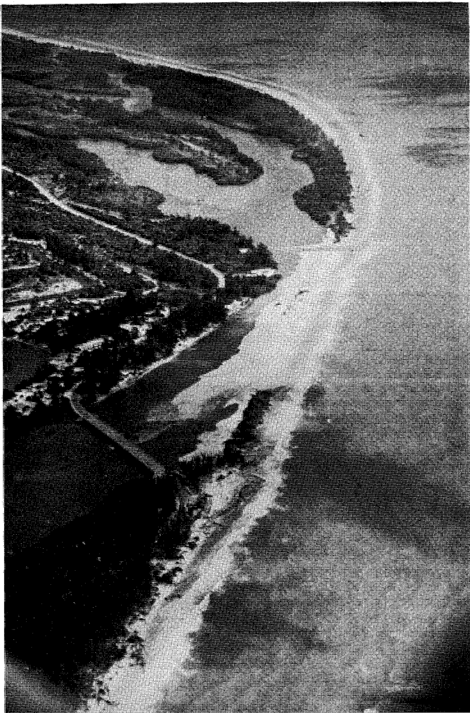
Turner Park --- or what's left of it -- on Captiva. Notice the new cut through Blind Pass; the erosion on the Gulf side, and the build-up in the pass itself.
