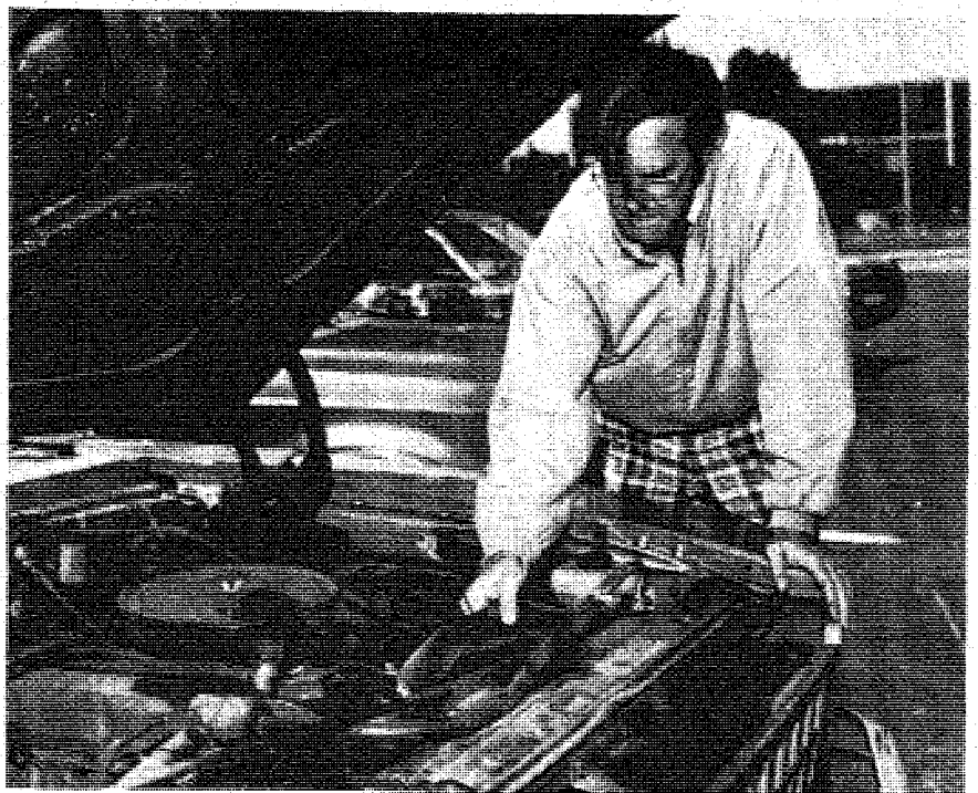
When checking radiator hoses, be certain the engine is cool. Should a hose be so deteriorated that it breaks, you're apt to get an unwanted bath of scalding radiator coolant. Checking hoses is just one step to take when making sure system is okay, says the Automotive Cooling System Institute.
